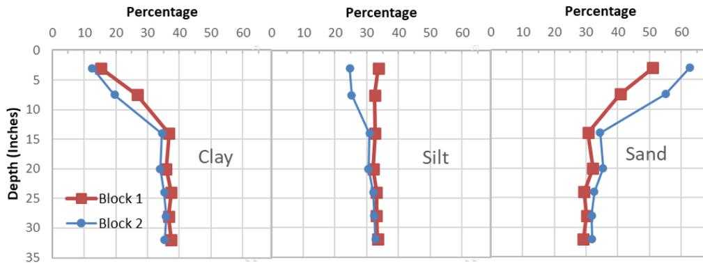
Figure 14. Soil texture observed at the South-West side (Block 1) and the North-East side (Block 2) of the LPD drain field, near the corresponding TDR sensors
