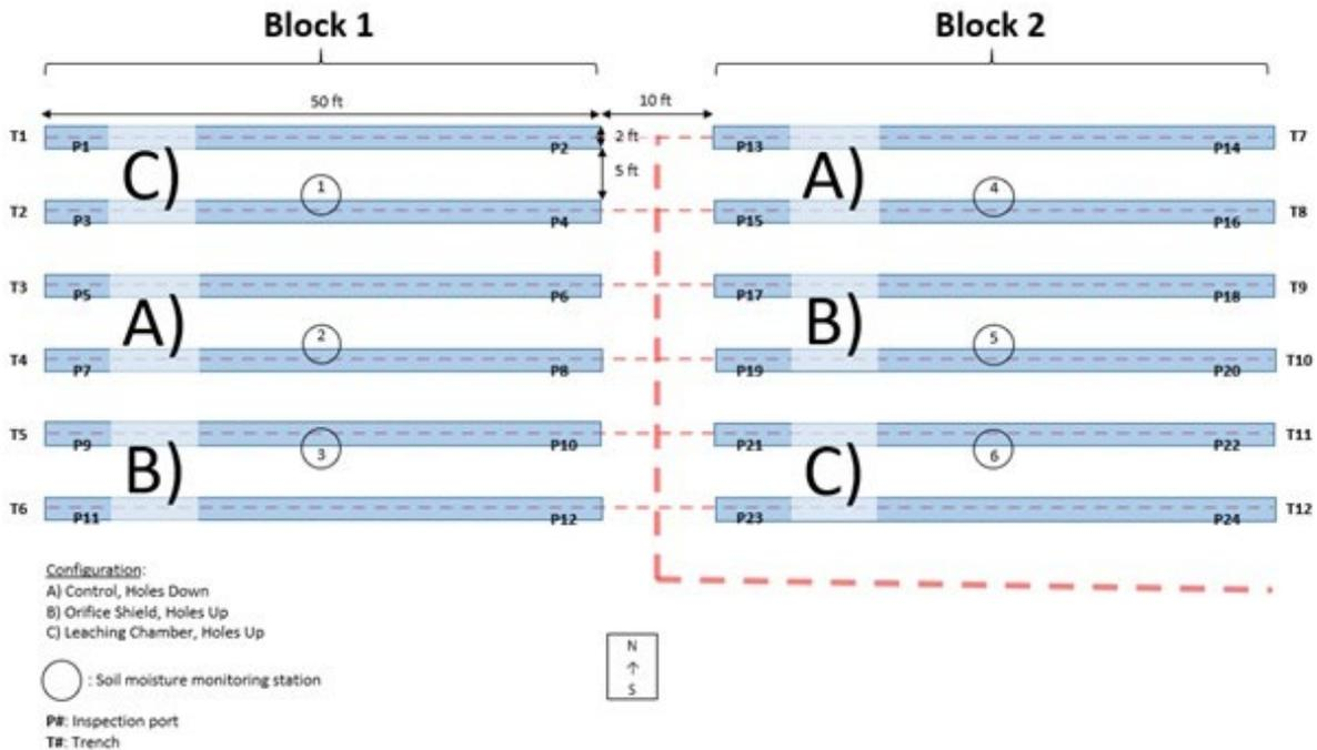
Figure 5. Details of experimental design for LPD project: Experimental design, location of TDR instrumentation installation, and location of inspection ports
