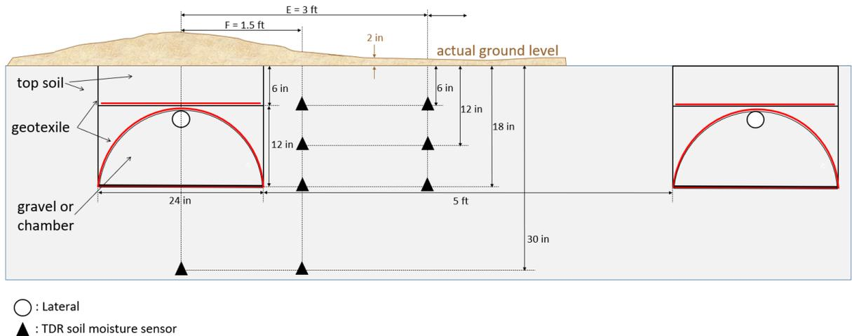
Figure 6. Details of experimental design for LPD project: Location of individual soil moisture monitoring sensors with respect to the trench section
