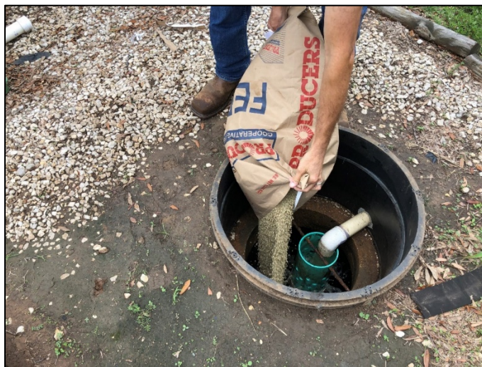
Figure 12- Adding grain-based animal feed to Feed Tank to raise BOD 5 concentration.
