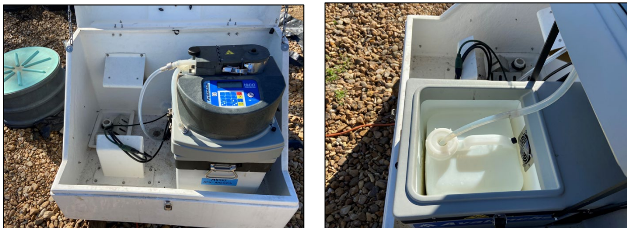
Figure 13- ISCO refrigerated sampler configured to deliver liquid amendments to ATU Pump Tank.
