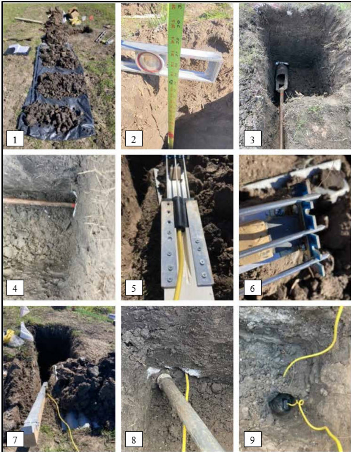
Figure 34. Phases of Time Domain Reflectometer (TDR) installation. Picture 1: 4-inches soil layers are removed and stored separately for later correct refilling of the hole; Picture 2: Depths are referred to a common ground level; Pictures 3-8: Installation of sensor below the trench; Picture 9: Sensor installed vertically at 30 inches of depth
