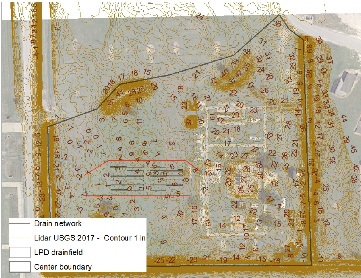
Figure 22. Location of the drainage relief network and Lidar USGS contour elevation lines (at 1 inch interval). Elevation is referred to the lowest point of the drain field (South West corner)
