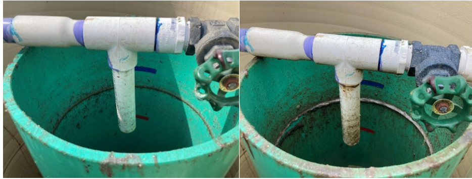
Figure 16. Detail of the calibration tank design. Left: at experiment start (with calibration tags); Right: at experiment end (noticeable the deposit where level has been controlled)
