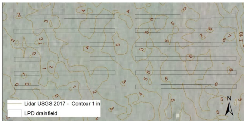
Figure 13. Lidar USGS contour elevation isolines (at 1 inch interval) in the drain field area. Elevation is referred to the lowest point (South West corner)
