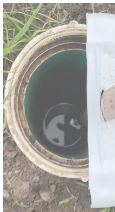
Figure 21. Inspection port monitoring consisted in the measurement of the distance between the port top and the water level, converted to water level based on elevation of the port top and the trench bottom
