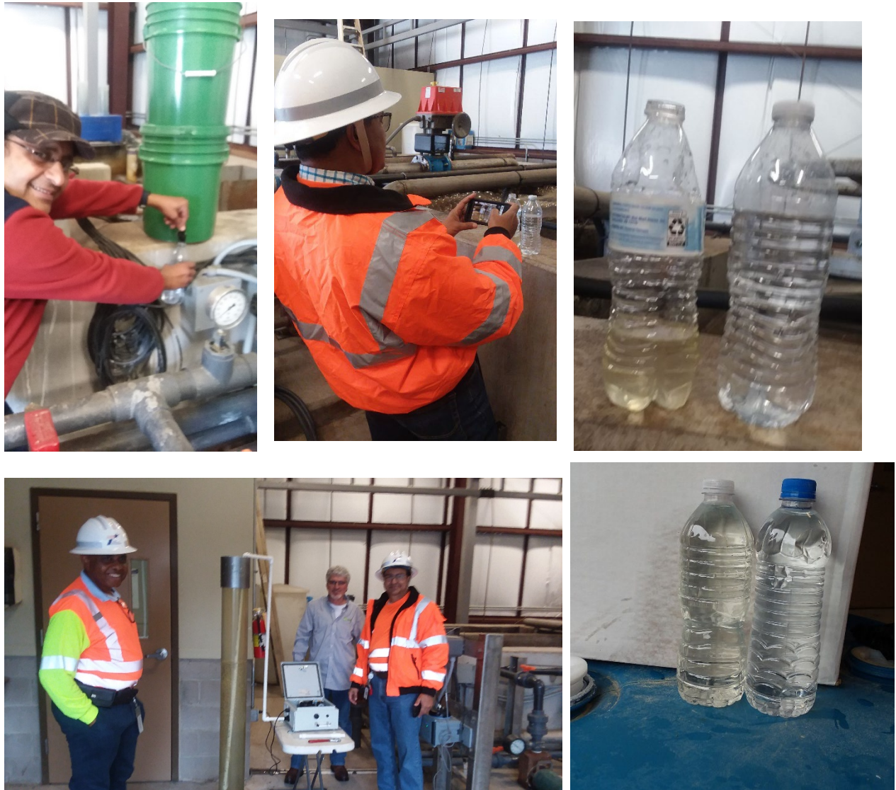
Photo 6: From top left to bottom right – field demonstration of charcoal filter (contained in the bottom green bucket) and ozonation (tall clear pipe in which ozone was pumped) to improve color of MBR effluent at the TxDOT wastewater reuse treatment plant.
