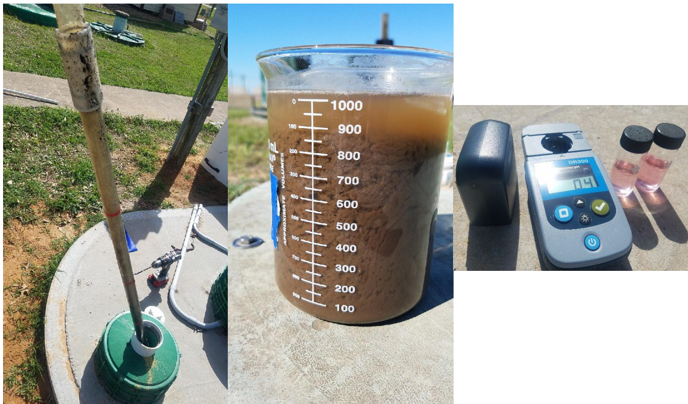
Photo 5: Sludge judge test for assessing sludge depth in trash-tank, settleability test for assessing sludge accumulation in aeration tank, and residual chlorine test to determine residual chlorine levels in the non-MBR system effluent. Sludge was not wasted during the experiment.
