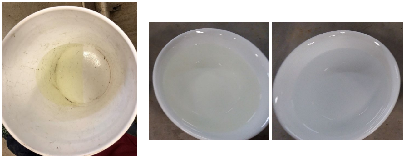
Photo 9: Left : The yellow color present in the MBR effluent was not adequate for reuse (Photo provided by TxDOT employee in November 2019). Middle : After of Ozone, and Right : After GAC filter (Middle and Right pictures taken in January 2022 by the PI during site visit; Ozone system has been installed, and TxDOT is in the process of installing GAC filter and chlorination systems)
