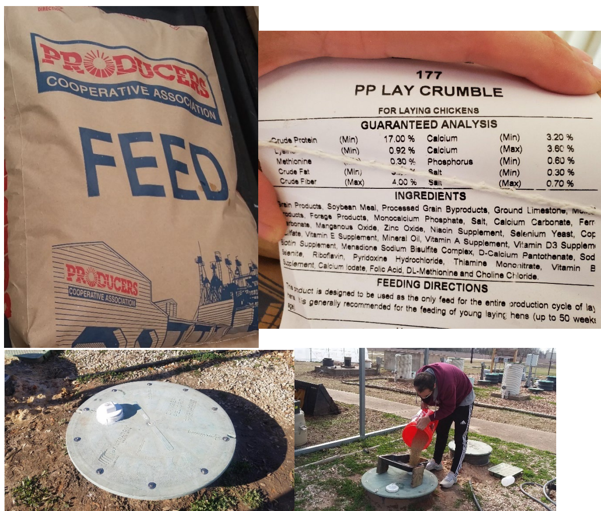
Photo 3: From top left to bottom right – 50 lb bag of FEED material, details on ingredients contained in the FEED material, tank lid modification for allowing easy access to add the FEED material daily, and finally Mesut adding the 10 lb of FEED material daily during the experiment.
