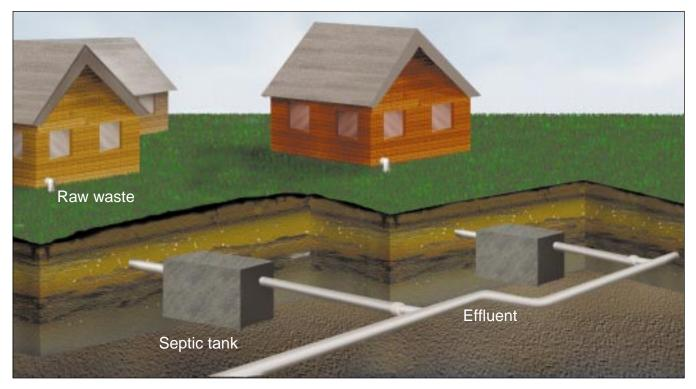
Figure 1: A small-diameter gravity sewer system.
