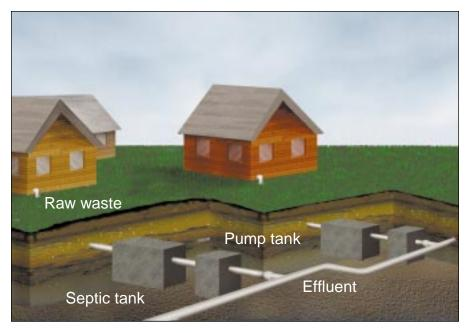
Figure 2: A septic tank effluent pump (STEP) system.
