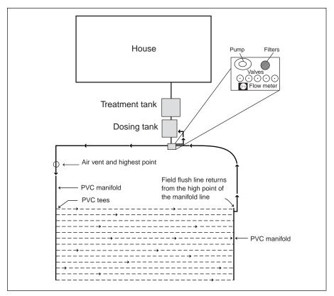
Figure 3: A drip distribution system for treatment and dispersal.
