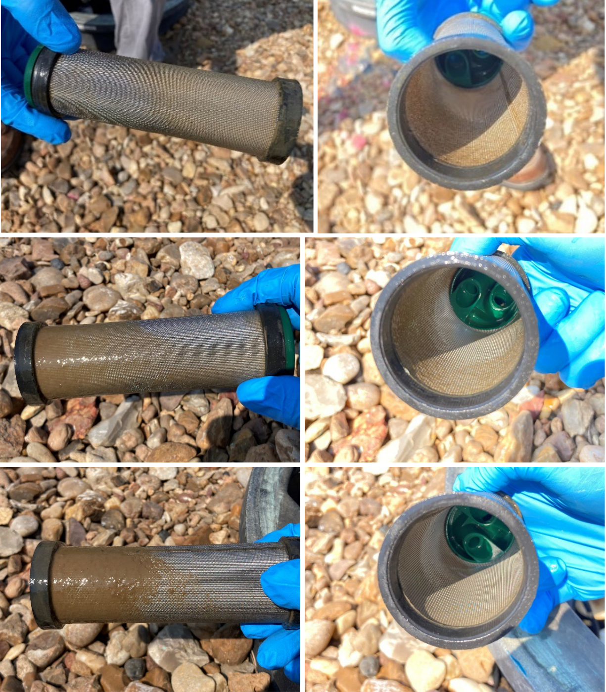
Figure 29. Filters status on August 25, 2023, after several days of sludge application: Simple screen (TOP), Aztec Dual Spin Filter #1 (MIDDLE), Aztec Dual Spin Filter #1 (BOTTOM).
