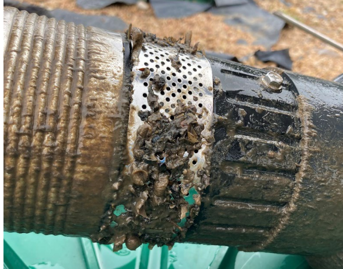
Figure 32. On November 2, 2023, sludge started to be collected from the trash tank (TOP). The flow and pressure declined during the dosing, likely due to the pump filter clogging (November 8, 2023, BOTTOM).
