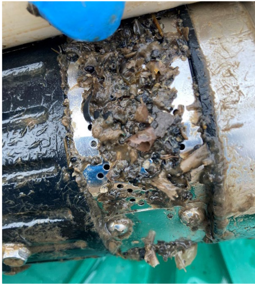
Figure 32. On November 2, 2023, sludge started to be collected from the trash tank (TOP). The flow and pressure declined during the dosing, likely due to the pump filter clogging (November 8, 2023, BOTTOM).
