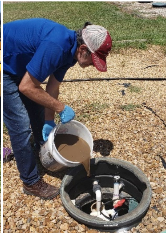
Figure 26. Sludge obtained from the MBR system and applied in the pump tanks (July 12, 2023).
