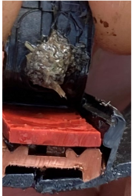
Figure 34. More deposit compared to the front or end of the line was found in middle sections (November 8, 2023). It is evident the deposit of some material inside the tubing, including inside the emitter.
