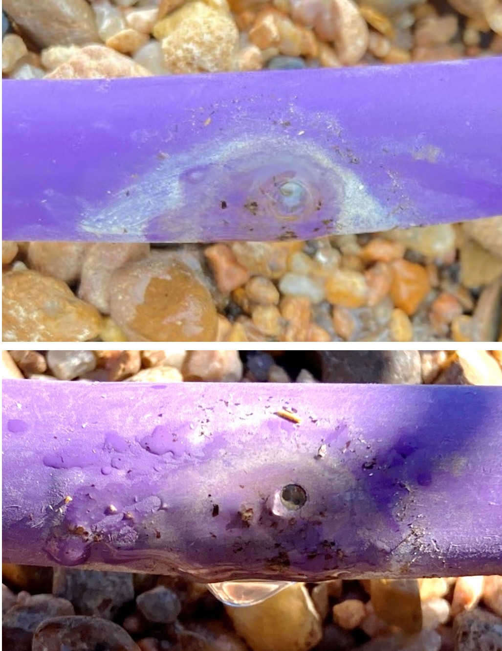
Figure 35. Some deposit was found outside the line, including larger material likely due to the type of sludge added in the last days (from the trash tank). Pictures were taken on the same portion of the line on November 11 (top) and on November 15 (bottom).
