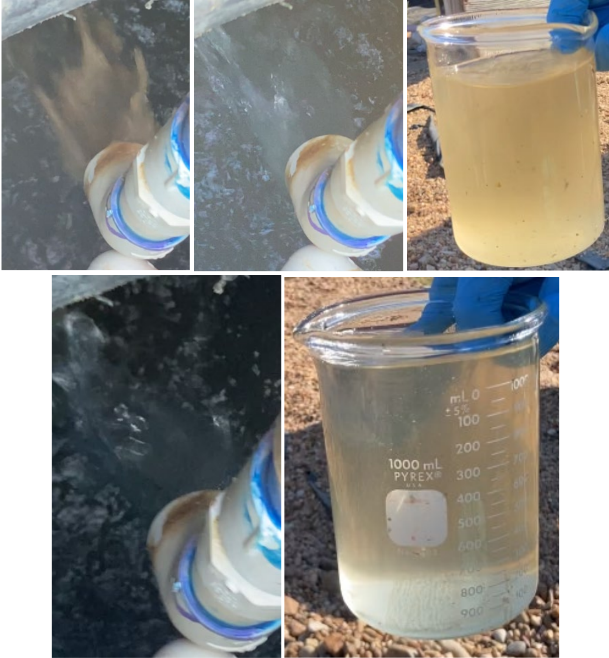
Figure 40. Visual comparison of samples collected from the return flow on September 7, 2023. Changing color progression and final sample from the Sc.A/D line (from top left to bottom right).
