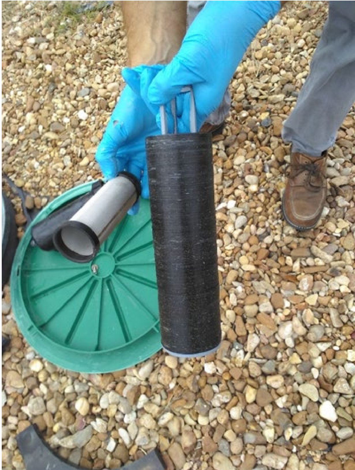
Figure 23. Disc filter compared to simple screen filter, at installation (September 22, 2023)
