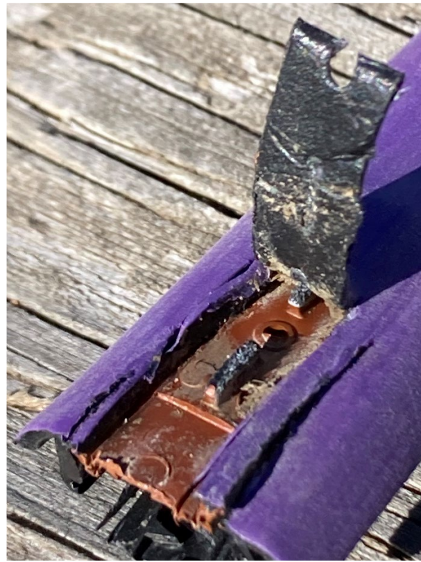
Figure 36. Simple screen filter line section on December 11, 2023. Line looked clean, likely because no sludge had been added for weeks in the last phases, and the line was flushed on November 7 and 8; emitters, on the other hand, showed signs of clogging, which was likely the reason for the flow constant decline.
