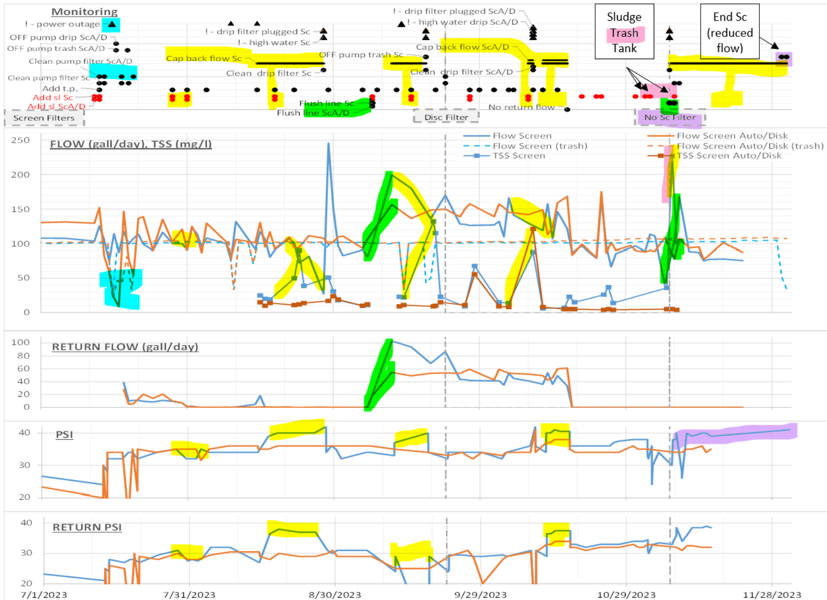
Figure 24. Details of monitoring and artificial clogging and issues. Colors are used here to highlight similar issues and consequences.
