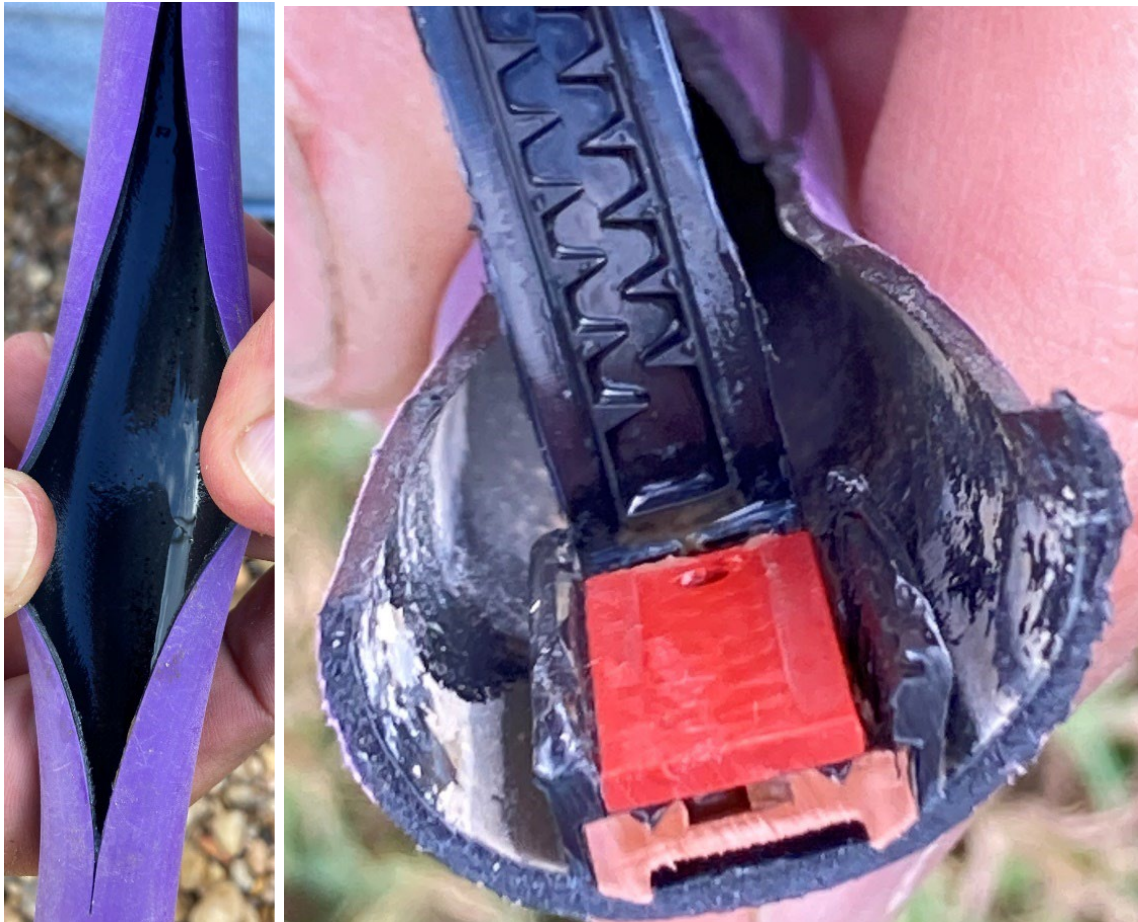
Figure 33. Drip line was cut open and observed toward the end of the experiment, right before the final clogging phases (November 8, 2023). Very little deposit was found in the end portions of the line, including in the emitters.
