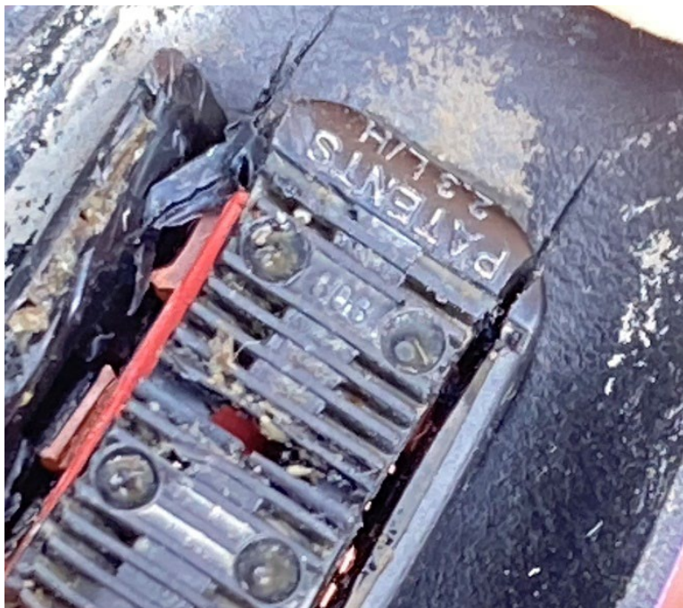
Figure 34. More deposit compared to the front or end of the line was found in middle sections (November 8, 2023). It is evident the deposit of some material inside the tubing, including inside the emitter.
