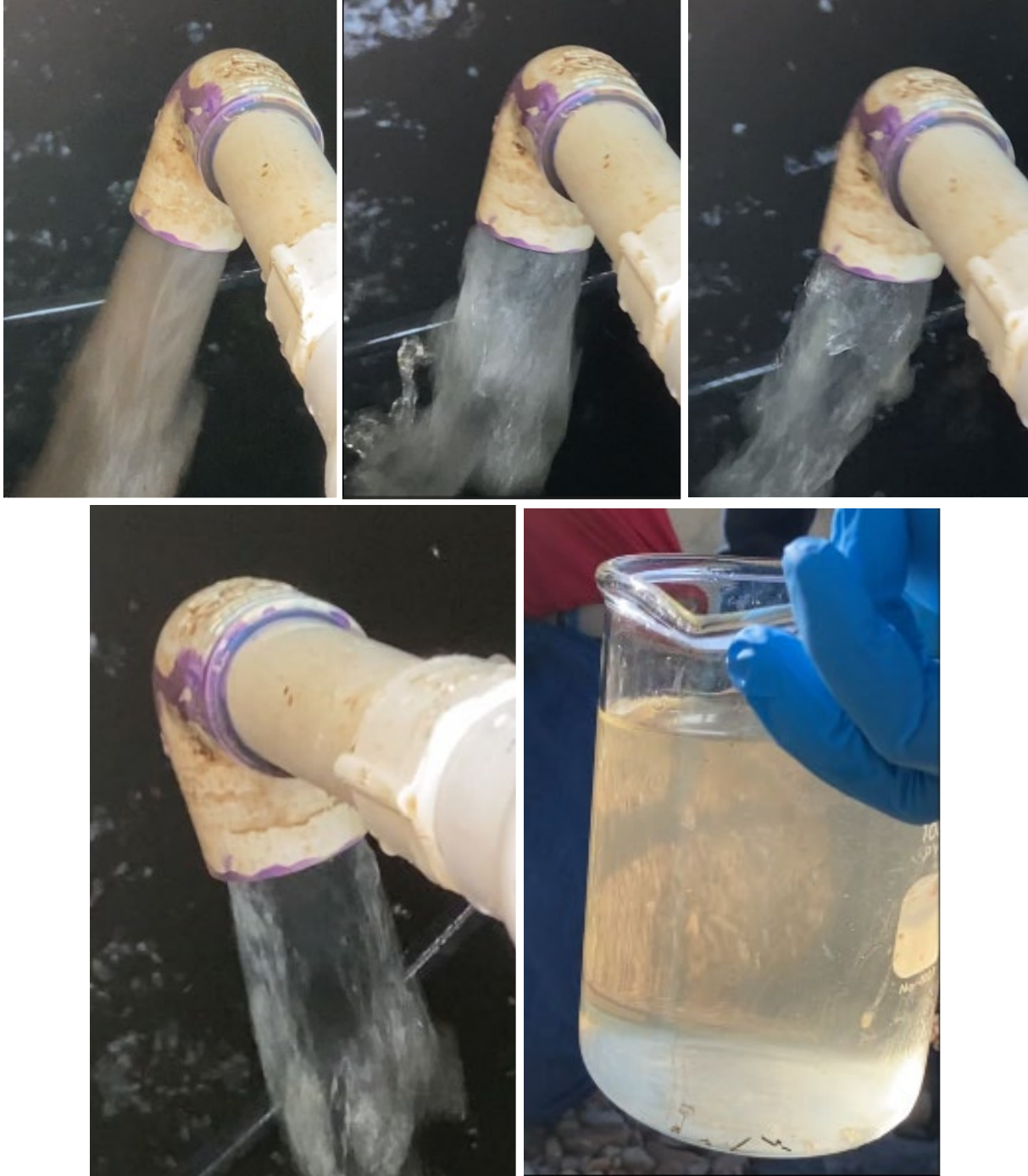
Figure 39. Visual comparison of samples collected from the return flow on September 7, 2023. Changing color progression and final sample from the Sc line (from top left to bottom right).
