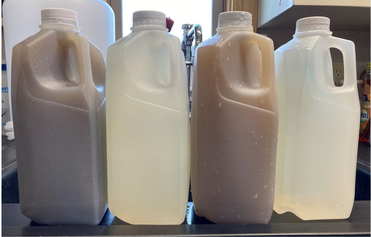
Figure 37. Visual comparison of samples collected from the pump tank bottom and from the return flow on July 28, 2023. From left to right: Sc pump, Sc return, Sc.A/D tank, Sc.A/D return.
