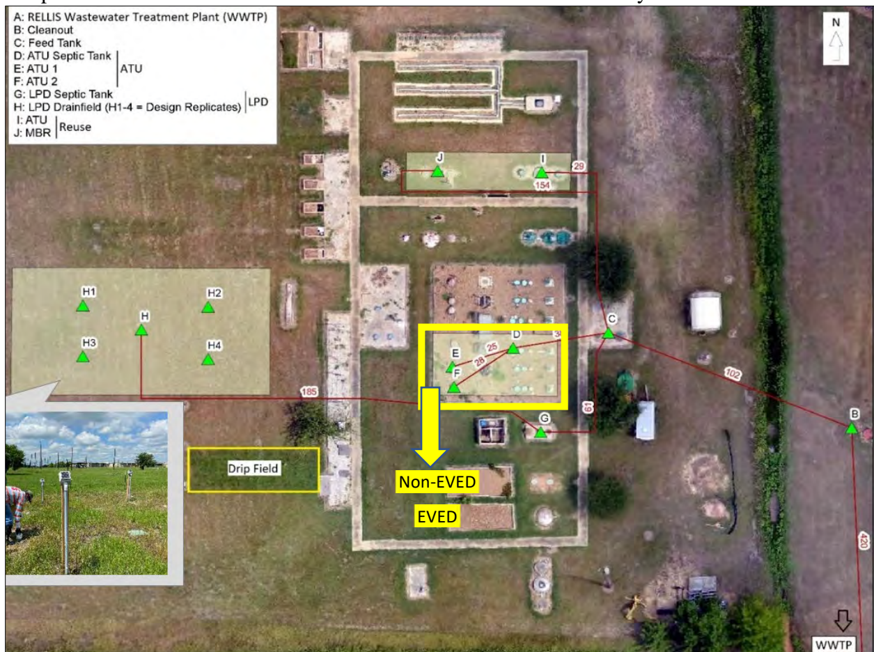
Figure 5: TAMU OSSF Center aerial view showing layout of the two ATUs, location of wetland cells used for evaluating performance of EVED and non-EVED systems and effluent flow line.
