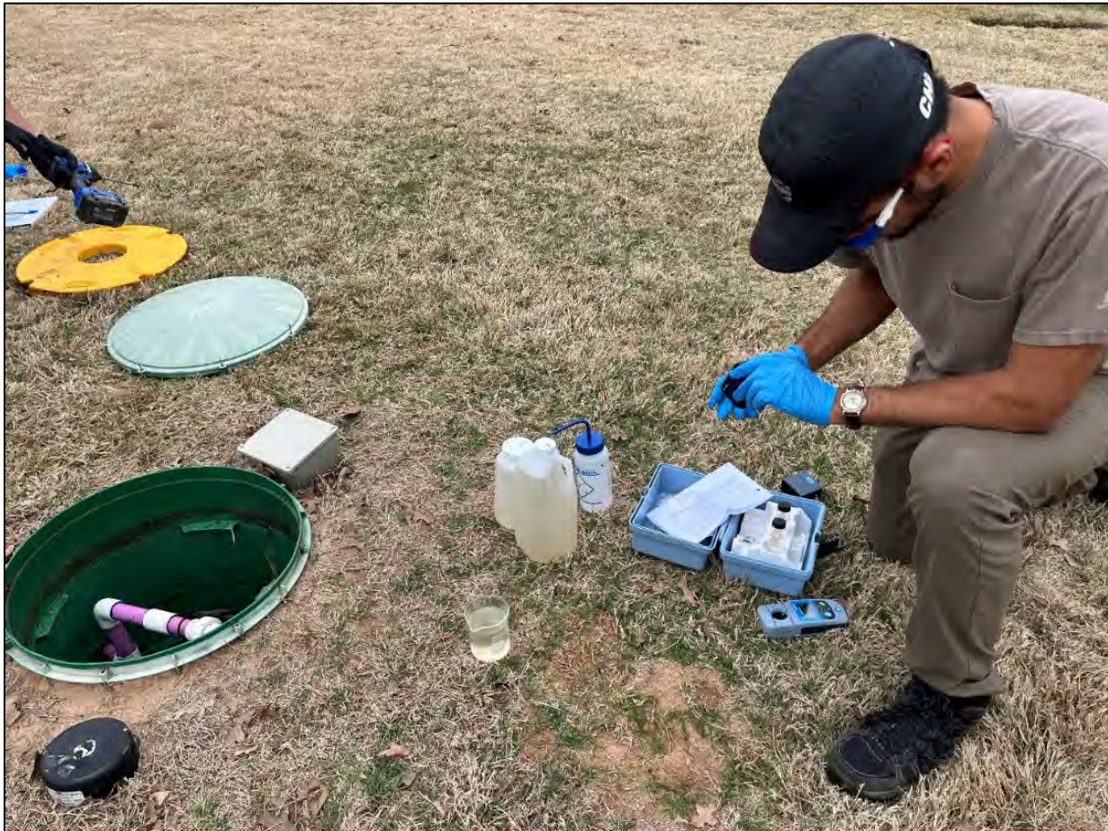
Figure 5- Measuring chlorine on-site at a residential ATU
