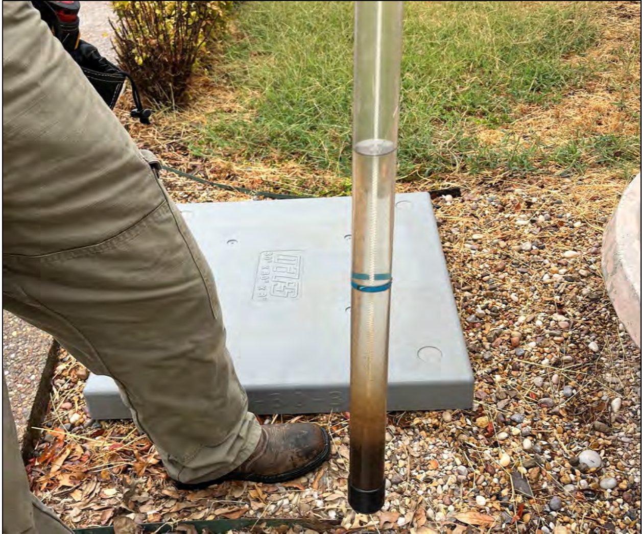
Figure 4 - Visually evaluating sludge level in residential ATU pump tank with sludge sampler
