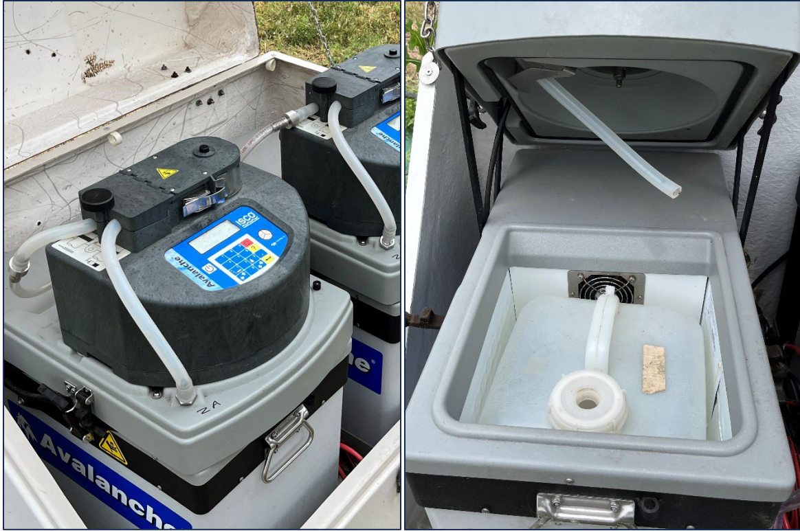
Figure 3. ISCO Avalanche refrigerated, programmable water sampler. Controller and pump (left), inside (right).
