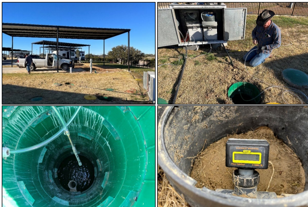
Figure 11. RV-5 Clockwise from top left; park overview, installing samplers, sampler intake strainer, and electronic flow meter.
