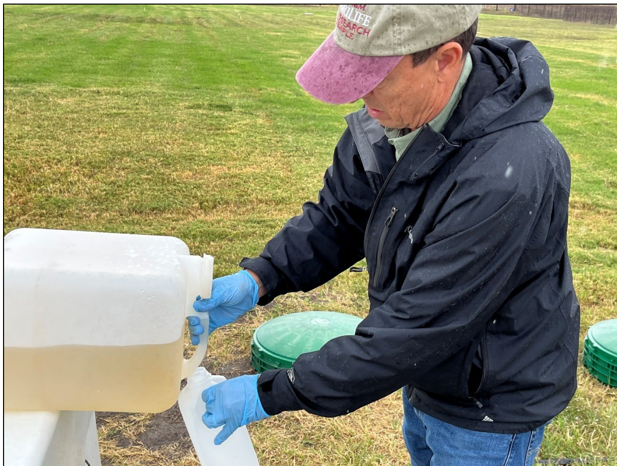
Figure 5. Collecting composite wastewater sample for laboratory BOD 5 and TSS analysis.
